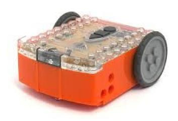
Michael: We are roadtesting V1 Edisons in Year 5 this term. The Edware programming language is very complicated, but they are working on Blockly and Python coding tools. v2 is supposed to have fixed the reliability problems with faulty gears and sticky wheels. Cheap, compatible with Lego, but not a huge fan.
