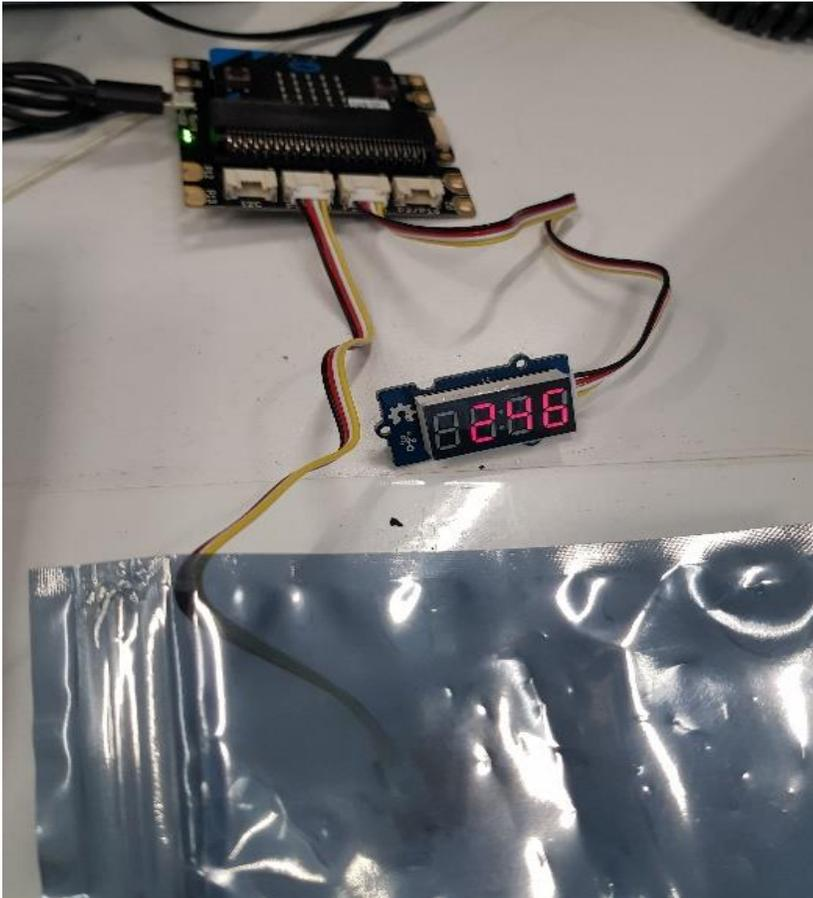
Hold over any material and gather data on how much light travels through the material.
